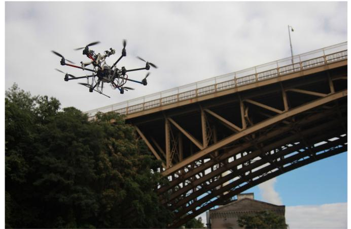
*Figure 1. The Aerial Robotic Infrastructure Analyst (ARIA) rapidly models critical infrastructure using small, low-flying robots. (Photo courtesy of Luke Yoder.)*
